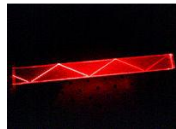
Total internal reflection of a light ray
