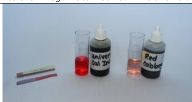
Litmus paper, universal indicator and red cabbage juice change colour in vinegar.
