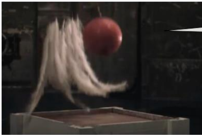
Figure 131 Photographs of a feather and a ball falling in a vacuum
