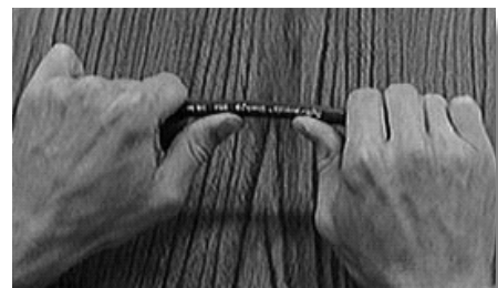
Do you have a broad, thick pencil? You'll find it's much harder to bend or break than an ordinary pencil.
