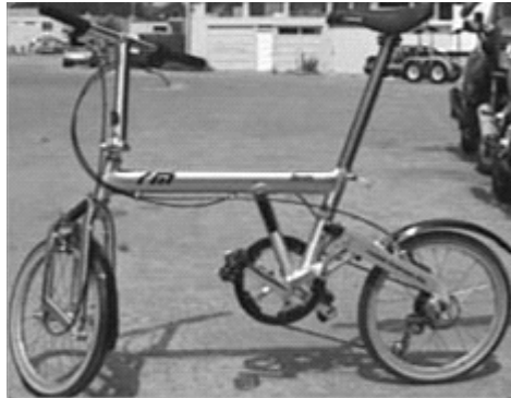
This folding bicycle has a very large diameter top tube, which helps give the bicycle strength.
