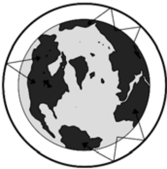
Radio waves reflecting off the ionosphere (the outer line) during skywave radio propagation
